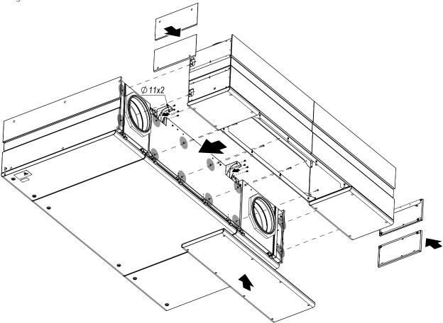
Install the decorative panels. Install the panels in the centre first, then the top and bottom panels. Special fasteners are used to mount the unit with the product. Mounting brackets for mounting the unit with the product are included with the unit.
