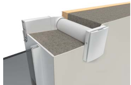
Angular mounting into a wall with standard thickness using KIT BlauPlast white 160 / KIT BlauPlast chrome 160
