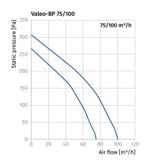
• The abrupt curves show high pressure performance and constant air flow of several **Valeo-BP** fans integrated into a single ventilation shaft.
