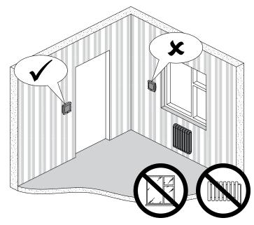
The installation place of the control panel must have stable temperatures and be not exposed to temperature fluctuations from heater batteries, vertical air convection, etc.
