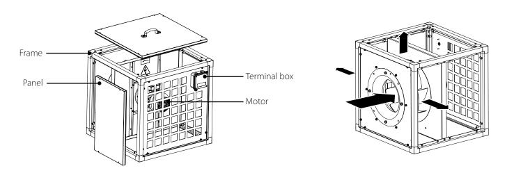
When connecting the fan to the air duct system, it is recommended to use the accessories specified in the User's manual. Connecting spigots can be of round cross-section.
