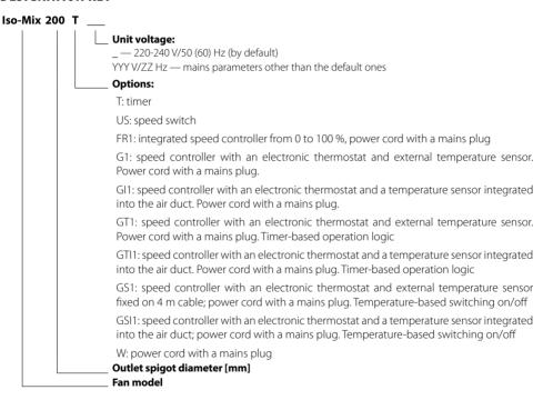
For a description of the fan options, see the «Electronics operation algorithm» section.
