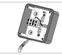
Connect the power cord wires to the terminal block and assemble the fan in reverse order. Supply power to the fan.
