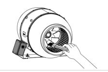
Connect an air duct on both sides of the fan. Supply power to the fan.
