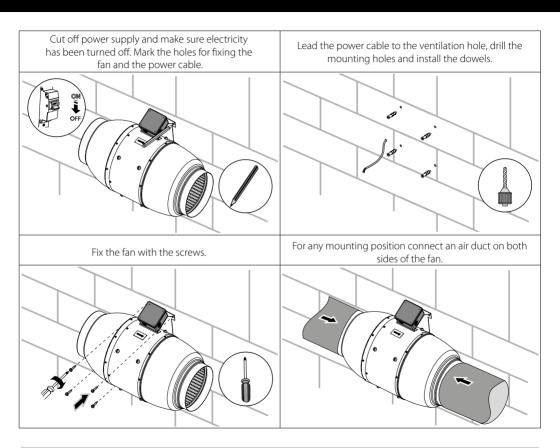
Cut off power supply and make sure electricity has been turned off. Remove the cover of the fan.
