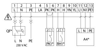
Connection of additional external control contacts is implemented in the control unit. For accessing the control unit open the unit door, release the screws fixing the shielding and remove it.
