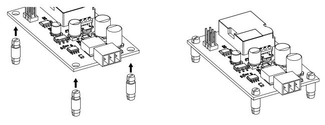
Install the sensor circuit board inside the unit in the bracket holes or in the wall at location specified in the user manual.
